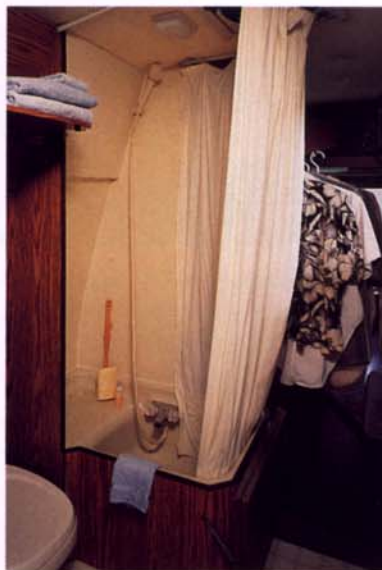
Combination shower/wardrobe gives you sit-down bathing facilities while maintaining valuable closet space. Just swing the wardrobe shelf and rack (with clothes still on hangers) out over the bed, fold down the tub cover and draw the curtain.
