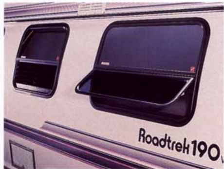
Awning windows provide superior air circulation even during foul weather. The Integrated Venting System provides effective yet inconspicuous ventilation of the refrigerator.
