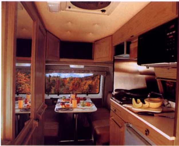
The galley is equipped with 3.0 cu.ft. refrigerator, microwave oven, LP gas stove, exhaust fan, sink and 6 feet of standing head room.
