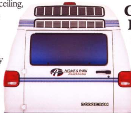
A 110V Fedders air conditioner built into the upper rear cabinets cools the interior while maintaining Roadtrek's aerodynamic shape and sleek roofline.
