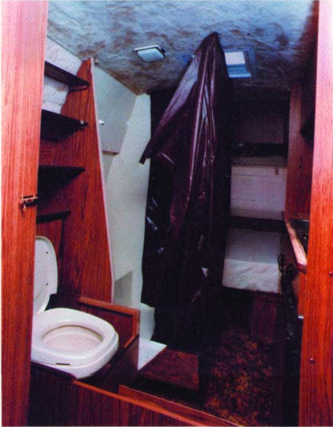
4' x 4' private washroom, 40" x 25" shower with fold away stall and sit-up tub in closet. To use shower simply pull and swing out coats on hangers, while they remain in place on rod fixed to shelf above, all together as one unit to rear over seat or bed. Next fold down shower pan and extend curtain, which is hanging stored behind coats on knobs at ceiling, forward to knobs in van centre.
